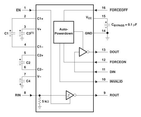
(1) C3 can be connected to  $V_{CC}$  or GND. NOTES: A. Resistor values shown are nominal.
