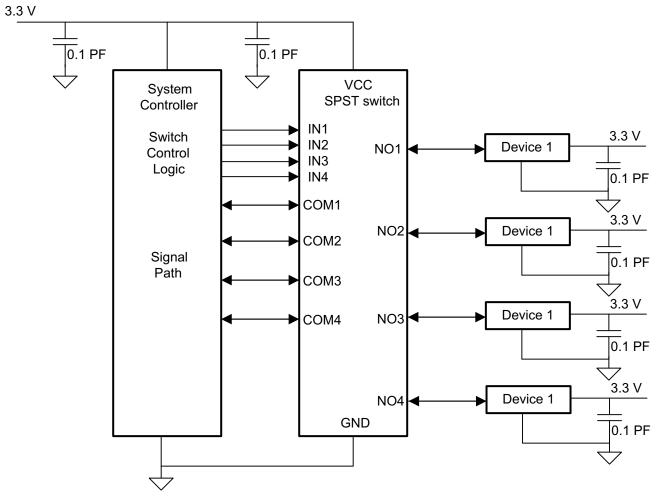
Figure 9. Typical Application Schematic
