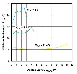
Figure 10. ON-State Resistance, R<sub>ON</sub> vs Analog Signal, V<sub>COM</sub>
