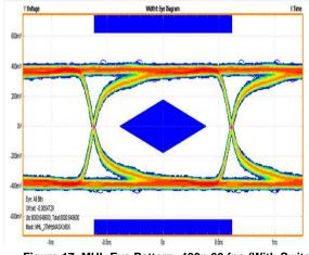
Figure 17. MHL Eye Pattern: 480p 60 fps (With Switch)
