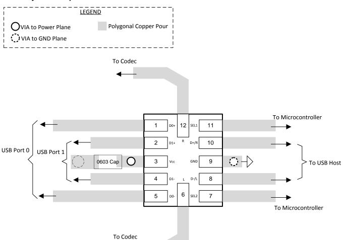
Figure 21. Layout Schematic
