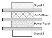
Figure 20. Four-Layer Board Stack-Up
