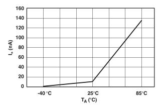
Figure 22. Power-Supply Current vs Temperature ( $V_{+} = 5 \text{ V}$ )
