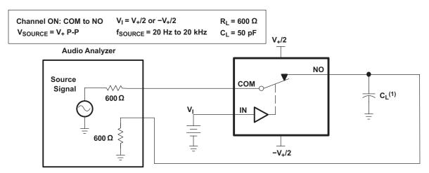
(1) C<sub>L</sub> includes probe and jig capacitance.
