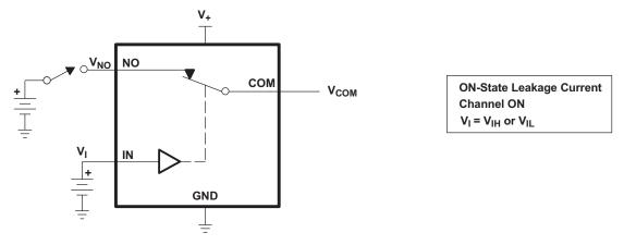
Figure 13. ON-State Leakage Current (I<sub>COM(ON)</sub>, I<sub>NC(ON)</sub>)
