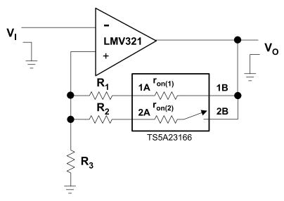
Figure 21. Gain-Control Circuit for OP Amplifier
