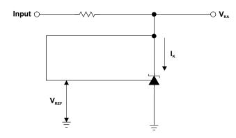
Figure 1. Test Circuit for  $V_{KA} = V_{REF}$
