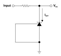
Figure 3. Test Circuit for I<sub>OFF</sub>
