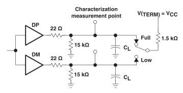
Figure 1. Differential Driver Switching Load
