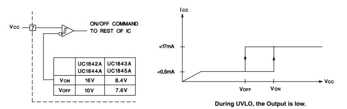
Figure 2. Under Voltage Lockout
