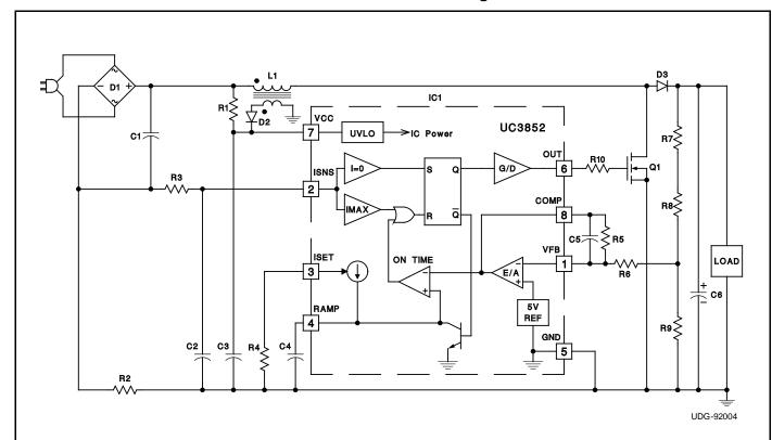
This circuit demonstrates a complete power factor preregulator based on the UC3852. This preregulator will supply up to 100 watts at 400VDC and exhibit power factor greater than 0.995 with less than 10% total harmonic distortion. Operating input range is 90V to 160V RMS at 50Hz to 60Hz.
