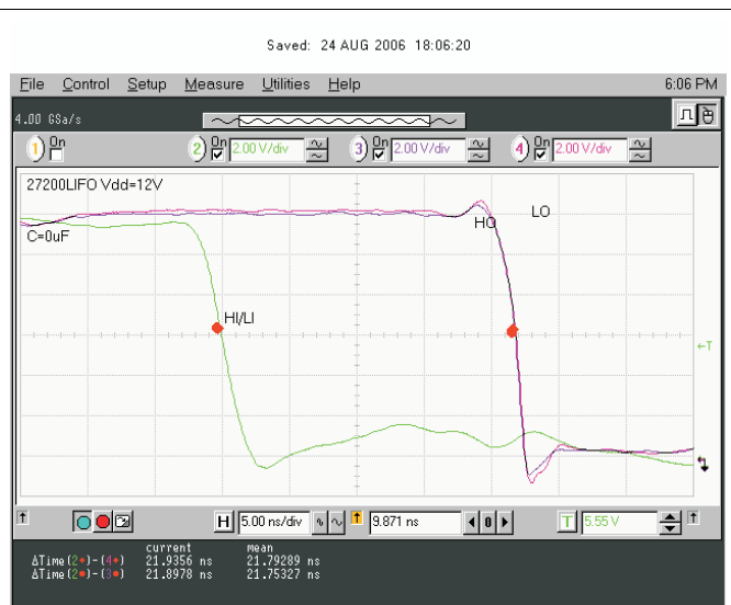
Figure 26. V_{LO} and V_{HO} Falling Edge Delay Matching
