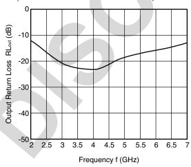
ANT2-RX OUTPUT RETURN LOSS vs. FREQUENCY (When TX-ANT1 and ANT2-RX are ON)
