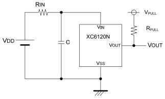
[Figure 1: Circuit connected with the input resistor]
