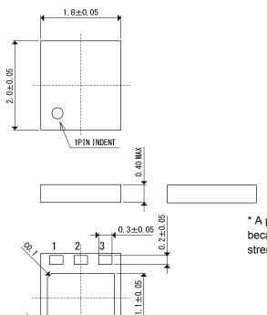
\* A part of the pin may appear from the side of the package because of it's structure, but reliability of the package and strength will not be changed below the standard.
