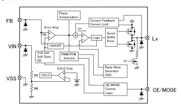
NOTE: The signal from CE/MODE Control Logic to PWM/PFM Selector is being fixed to "L" level inside, and XC9235 series chooses only PWM control.
