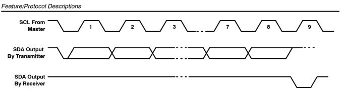
Figure 3–9. Serial-Bus Protocol Acknowledge
