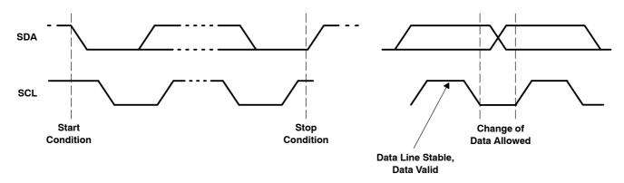
Figure 3–8. Serial-Bus Start/Stop Conditions and Bit Transfers
