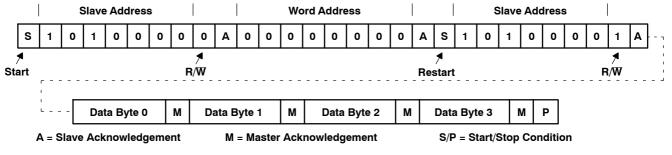
Figure 3–12. Serial-Bus Protocol—Multibyte Read
