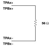
Figure 11–1. Test Load Diagram
