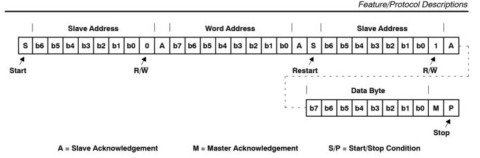
Figure 3–11. Serial-Bus Protocol—Byte Read
