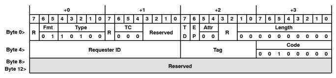
Figure 3–5 and Figure 3–6 illustrate the format for both the assert and deassert INTA messages.
