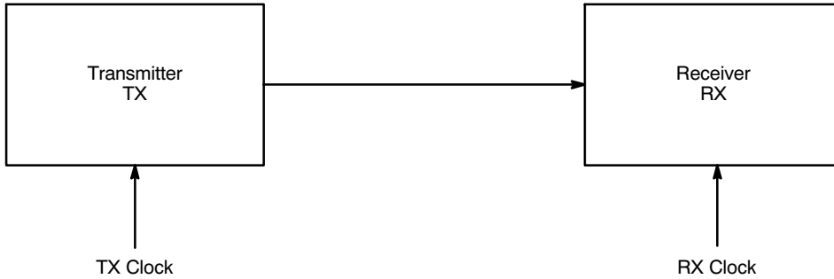
Figure 33. Example of a Serial Data Transmission System
