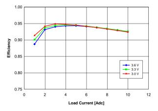
Fig. 2.0V.4: Efficiency vs. load current and input voltage for Vout = 2.0 V converter mounted vertically with air flowing at a rate of 200 LFM (1 m/s) and Ta = 25 °C.
