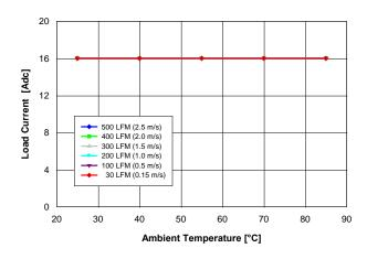
Fig. 1.2V.2: Available load current vs. ambient temperature and airflow rates for Vout = 1.2 V converter mounted horizontally with Vin = 5 V, and maximum MOSFET temperature ≤ 120 °C.
