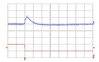
Fig. 3.3V.8: Output voltage response for Vout = 3.3 V to negative load current step change from 10 A to 5 A with slew rate of -5 A/μs at Vin = 5 V. Top trace: output voltage (100 mV/div.); Bottom trace: load current (5 A/div.). Co = 47 μF ceramic + 1 μF ceramic. Time scale: 20 μs/div.
