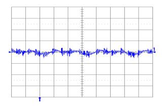
Fig. 1.0V.6: Output voltage ripple (20 mV/div.) at full rated load current into a resistive load with external capacitance 47 μF ceramic + 1 μF ceramic, and Vin = 5 V for Vout = 1.0 V.
