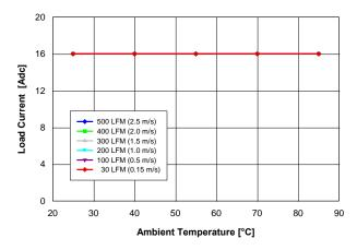
Fig. 2.5V.2: Available load current vs. ambient temperature and airflow rates for Vout = 2.5 V converter mounted horizontally with Vin = 5 V, and maximum MOSFET temperature ≤ 120 °C.
