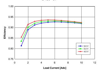
Fig. 2.0V.3: Efficiency vs. load current and input voltage for Vout = 2.0 V converter mounted vertically with air flowing at a rate of 200 LFM (1 m/s) and Ta = 25 °C.
