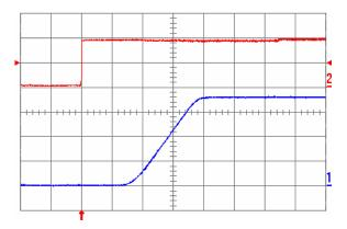
Fig. 1.8V.5: Turn-on transient for Vout = 1.8 V with the application of Enable signal at full rated load current (resistive) and 47 μF external capacitance at Vin = 5 V. Top trace: Enable signal (2 V/div.); Bottom trace: output voltage (500 mV/div.); Time scale: 2 ms/div.
