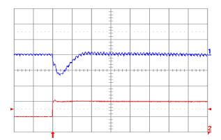
Fig. 1.5V.7: Output voltage response for Vout = 1.5 V to positive load current step change from 5 A to 10 A with slew rate of 5 A/μs at Vin = 5V. Top trace: output voltage (100 mV/div.); Bottom trace: load current (5 A/div.). Co = 47 μF ceramic + 1 μF ceramic. Time scale: 20 μs/div.
