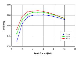
Fig. 0.7525V.3: Efficiency vs. load current and input voltage for Vout = 0.7525 V converter mounted vertically with air flowing at a rate of 200 LFM (1 m/s) and Ta = 25 °C.
