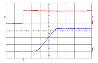
Fig. 3.3V.5: Turn-on transient for Vout = 3.3 V with the application of Enable signal at full rated load current (resistive) and 47 μF external capacitance at Vin = 5 V. Top trace: Enable signal (2 V/div.); Bottom trace: output voltage (1 V/div.); Time scale: 2 ms/div.
