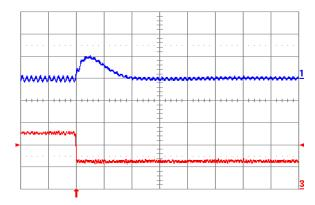
Fig. 1.0V.8: Output voltage response for Vout = 1.0 V to negative load current step change from 10 A to 5 A with slew rate of -5 A/μs at Vin = 5 V. Top trace: output voltage (100 mV/div.); Bottom trace: load current (5 A/div.). Co = 47 μF ceramic + 1 μF ceramic. Time scale: 20 μs/div.
