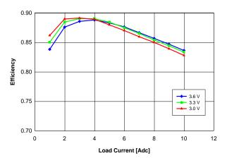
Fig. 0.7525V.4: Efficiency vs. load current and input voltage for Vout = 0.7525 V converter mounted vertically with air flowing at a rate of 200 LFM (1 m/s) and Ta = 25 °C.
