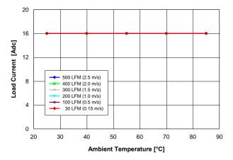
Fig. 1.0V.1: Available load current vs. ambient temperature and airflow rates for Vout = 1.0 V converter mounted vertically with Vin = 5 V, and maximum MOSFET temperature ≤ 120 °C.
