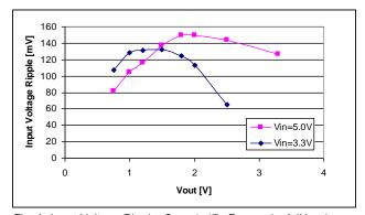
Fig. A: Input Voltage Ripple,  $C_{IN} = 4x47 \,\mu\text{F}$  ceramic, full load.
