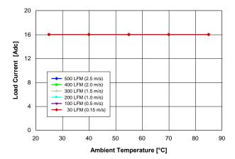
Fig. 0.7525V.2: Available load current vs. ambient temperature and airflow rates for Vout = 0.7525 V converter mounted horizontally with Vin = 5 V, and maximum MOSFET temperature  $\leq$  120  $^{\circ}$ C.
