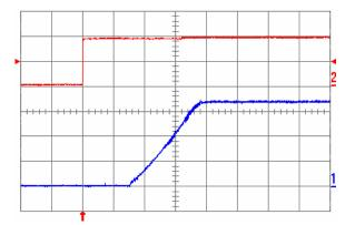
Fig. 0.7525V.5: Turn-on transient for Vout = 0.7525 V with the application of Enable signal at full rated load current (resistive) and 47 μF external capacitance at Vin = 5 V. Top trace: Enable signal (2 V/div.); Bottom trace: output voltage (200 mV/div.); Time scale: 2 ms/div.
