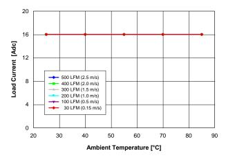
Fig. 1.8V.2: Available load current vs. ambient temperature and airflow rates for Vout = 1.8 V converter mounted horizontally with Vin = 5 V, and maximum MOSFET temperature ≤ 120 °C.
