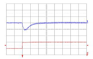
Fig. 2.0V.7: Output voltage response for Vout = 2.0 V to positive load current step change from 5 A to 10 A with slew rate of 5 A/μs at Vin = 5 V. Top trace: output voltage (100 mV/div.); Bottom trace: load current (5 A/div.). Co = 47 μF ceramic + 1 μF ceramic. Time scale: 20 μs/div.
