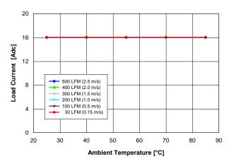
Fig. 3.3V.2: Available load current vs. ambient temperature and airflow rates for Vout = 3.3 V converter mounted horizontally with Vin = 5 V, and maximum MOSFET temperature ≤ 120 °C.
