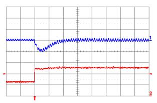
Fig. 1.0V.7: Output voltage response Vout = 1.0 V to positive load current step change from 5 A to 10 A with slew rate of 5 A/ $\mu$ s at Vin = 5 V. Top trace: output voltage (100 mV/div.); Bottom trace: load current (5 A/div.). Co = 47  $\mu$ F ceramic + 1  $\mu$ F ceramic. Time scale: 20  $\mu$ s/div.
