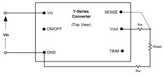
Fig. D: Remote sense circuit configuration.
