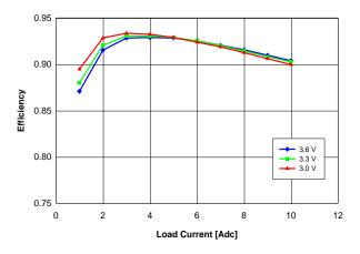
Fig. 1.5V.4: Efficiency vs. load current and input voltage for Vout = 1.5 V converter mounted vertically with air flowing at a rate of 200 LFM (1 m/s) and Ta = 25 °C.
