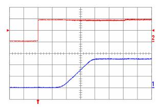
Fig. 2.5V.5: Turn-on transient for Vout = 2.5 V with the application of Enable signal at full rated load current (resistive) and 47 μF external capacitance at Vin = 5 V. Top trace: Enable signal (2 V/div.); Bottom trace: output voltage (1 V/div.); Time scale: 2 ms/div.
