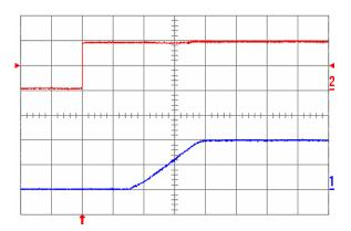
Fig. 1.0V.5: Turn-on transient for Vout = 1.0 V with the application of Enable signal at full rated load current (resistive) and 47 μF external capacitance at Vin = 5 V. Top trace: Enable signal (2 V/div.); Bottom trace: output voltage (500 mV/div.); Time scale: 2 ms/div.
