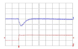
Fig. 1.2V.6: Output voltage response for Vout = 1.2 V to positive load current step change from 5 A to 10 A with slew rate of 5 A/μs at Vin = 5 V. Top trace: output voltage (100 mV/div.); Bottom trace: load current (5 A/div.). Co = 47 μF ceramic + 1 μF ceramic. Time scale: 20 μs/div.
