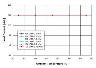
Fig. 2.5V.1: Available load current vs. ambient temperature and airflow rates for Vout = 2.5 V converter mounted vertically with Vin = 5 V, and maximum MOSFET temperature  $\leq 120 \text{ °C}$ .
