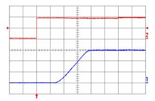
Fig. 1.5V.5: Turn-on transient for Vout = 1.5 V with the application of Enable signal at full rated load current (resistive) and 47 μF external capacitance at Vin = 5 V. Top trace: Enable signal (2 V/div.); Bottom trace: output voltage (500 mV/div.); Time scale: 2 ms/div.
