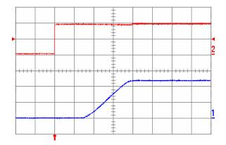
Fig. 1.2V.5: Turn-on transient for Vout = 1.2 V with the application of Enable signal at full rated load current (resistive) and 47 μF external capacitance at Vin = 5 V. Top trace: Enable signal (2 V/div.); Bottom trace: output voltage (500 mV/div.); Time scale: 2 ms/div.
