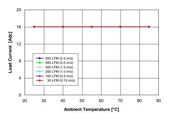
Fig. 2.0V.2: Available load current vs. ambient temperature and airflow rates for Vout = 2.0 V converter mounted horizontally with Vin = 5 V, and maximum MOSFET temperature ≤ 120 °C.
