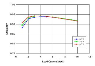
Fig. 1.8V.4: Efficiency vs. load current and input voltage for Vout = 1.8 V converter mounted vertically with air flowing at a rate of 200 LFM (1 m/s) and Ta = 25 °C.
