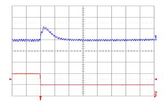
Fig. 2.5V.8: Output voltage response for Vout = 2.5 V to negative load current step change from 10 A to 5 A with slew rate of -5 A/μs at Vin = 5 V. Top trace: output voltage (100 mV/div.); Bottom trace: load current (5 A/div.). Co = 47 μF ceramic + 1 μF ceramic. Time scale: 20 μs/div.
