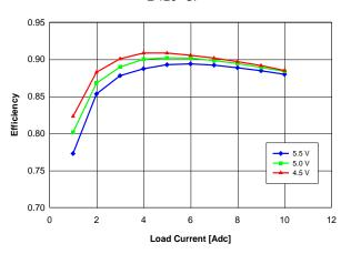
Fig. 1.2V.3: Efficiency vs. load current and input voltage for Vout = 1.2 V converter mounted vertically with air flowing at a rate of 200 LFM (1 m/s) and Ta = 25 °C.
