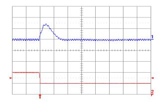
Fig. 2.0V.8: Output voltage response for Vout = 2.0 V to negative load current step change from 10 A to 5 A with slew rate of -5 A/μs at Vin = 5 V. Top trace: output voltage (100 mV/div.); Bottom trace: load current (5 A/div.). Co = 47 μF ceramic + 1 μF ceramic. Time scale: 20 μs/div.
