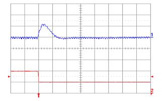
Fig. 1.5V.8: Output voltage response for Vout = 1.5 V to negative load current step change from 10 A to 5 A with slew rate of -5 A/μs at Vin = 5 V. Top trace: output voltage (100 mV/div.); Bottom trace: load current (5 A/div.). Co = 47 μF ceramic + 1 μF ceramic. Time scale: 20 μs/div.
