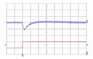
Fig. 3.3V.7: Output voltage for Vout = 3.3 V to positive load current step change from 5 A to 10 A with slew rate of 5 A/μs at Vin = 5 V. Top trace: output voltage (100 mV/div.); Bottom trace: load current (5 A/div.). Co = 47 μF ceramic + 1 μF ceramic. Time scale: 20 μs/div.
