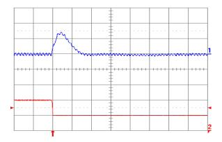
Fig. 1.8V.8: Output voltage response for Vout = 1.8 V to negative load current step change from 10 A to 5 A with slew rate of -5 A/μs at Vin = 5 V. Top trace: output voltage (100 mV/div.); Bottom trace: load current (5 A/div.). Co = 47 μF ceramic + 1 μF ceramic. Time scale: 20 μs/div.
