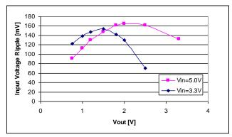
Fig. B: Input Voltage Ripple, CIN = 470  $\mu$ F polymer + 2 x 47  $\mu$ F ceramic.
