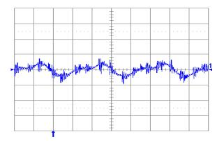
Fig. 2.5V.6: Output voltage ripple (20 mV/div.) at full rated load current into a resistive load with external capacitance 47 μF ceramic + 1 μF ceramic, and Vin = 5 V for Vout = 2.5 V.
