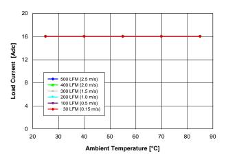
Fig. 2.0V.1: Available load current vs. ambient temperature and airflow rates for Vout = 2.0 V converter mounted vertically with Vin = 5 V, and maximum MOSFET temperature  $\leq 120 \text{ °C}$ .
