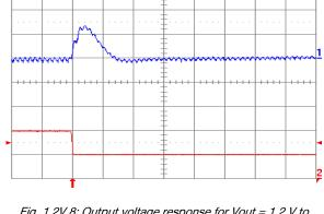
Fig. 1.2V.8: Output voltage response for Vout = 1.2 V to negative load current step change from 10 A to 5 A with slew rate of -5 A/μs at Vin = 5 V. Top trace: output voltage (100 mV/div.); Bottom trace: load current (5 A/div.). Co = 47 μF ceramic + 1 μF ceramic. Time scale: 20 μs/div.
