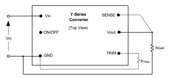
Fig. E: Configuration for programming output voltage.
