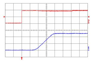
Fig. 2.5V.5: Turn-on transient for Vout = 2.5 V with the application of Enable signal at full rated load current (resistive) and 47 μF external capacitance at Vin = 5 V. Top trace: Enable signal (2 V/div.); Bottom trace: output voltage (1 V/div.); Time scale: 2 ms/div.
