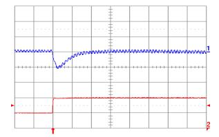
Fig. 2.5V.7: Output voltage response for Vout = 2.5 V to positive load current step change from 5 A to 10 A with slew rate of 5 A/μs at Vin = 5 V. Top trace: output voltage (100 mV/div.); Bottom trace: load current (5 A/div.). Co = 47 μF ceramic + 1 μF ceramic. Time scale: 20 μs/div.
