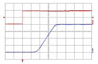
Fig. 2.0V.5: Turn-on transient for Vout = 2.0 V with the application of Enable signal at full rated load current (resistive) and 47 μF external capacitance at Vin = 5 V. Top trace: Enable signal (2 V/div.); Bottom trace: output voltage (500 mV/div.); Time scale: 2 ms/div.
