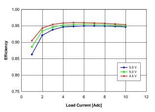
Fig. 3.3V.3: Efficiency vs. load current and input voltage for Vout = 3.3 V converter mounted vertically with air flowing at a rate of 200 LFM (1 m/s) and Ta = 25 °C.
