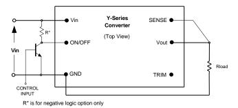
Fig. C: Circuit configuration for ON/OFF function.
