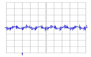
Fig. 2.0V.6: Output voltage ripple (20 mV/div.) at full rated load current into a resistive load with external capacitance  $47 \,\mu\text{F}$  ceramic +  $1 \,\mu\text{F}$  ceramic, and Vin =  $5 \,\text{V}$  for Vout =  $2.0 \,\text{V}$ . Time scale:  $2 \,\mu\text{S}/\text{div}$
