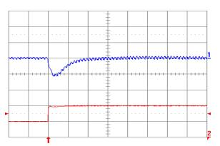
Fig. 1.8V.7: Output voltage response for Vout = 1.8 V to positive load current step change from 5 A to 10 A with slew rate of 5 A/μs at Vin = 5 V. Top trace: output voltage (100 mV/div.); Bottom trace: load current (5 A/div.). Co = 47 μF ceramic + 1 μF ceramic. Time scale: 20 μs/div.
